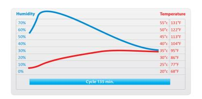
Test with an ambient temperature of 25°C / 77°F and a humidity of 60%.
